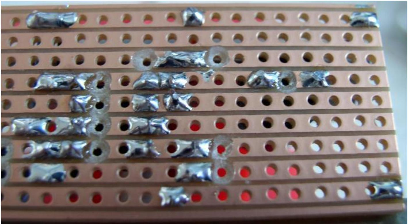
The final completed amplifier circuit with a short length of screened cable (grey) leading off to the volume control.
