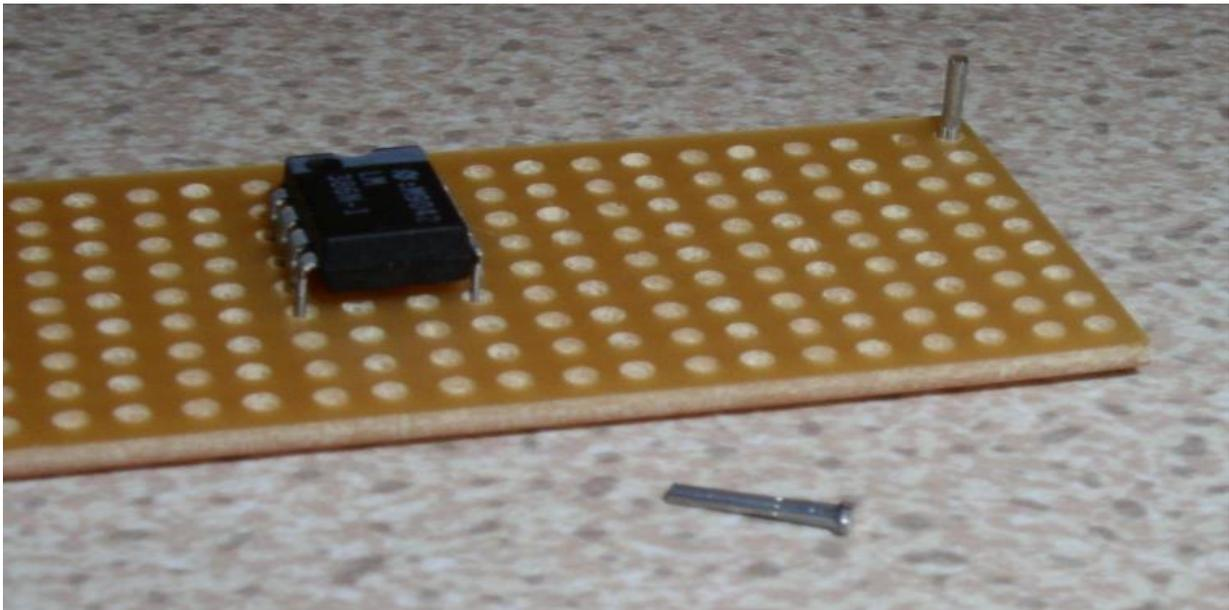
A veropin is shown above (centre bottom). Push two veropins through the copper side at the right hand side on track extremities. It is a good idea to separate power supply rails by at least one vero track.
