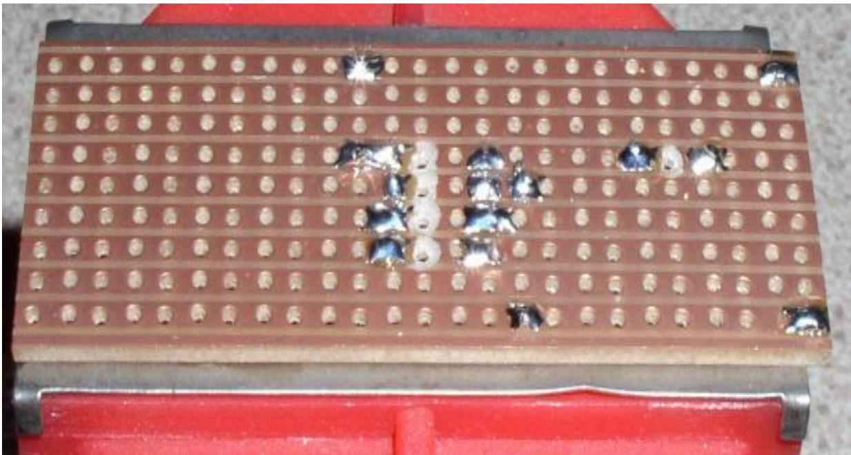
As the output capacitor has been soldered, the zobel network comprising of the 1R5 resistor and 100nF capacitor are wired up. Referring to the schematic, one end of the resistor is also connected to pin 5, one end of the capacitor goes to ground, and the free ends of these two components are wired together.
