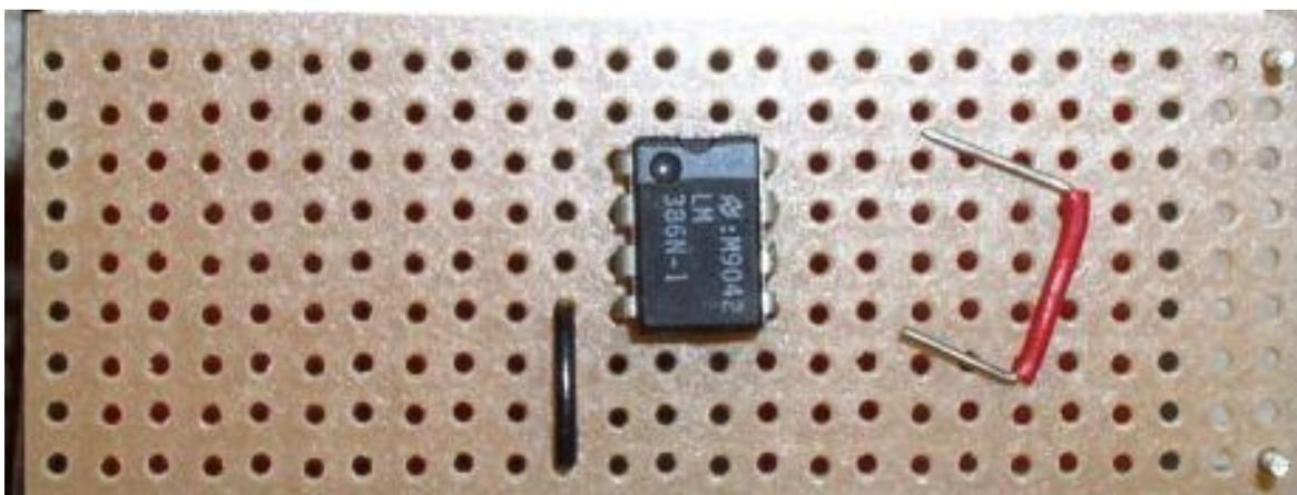
The wire (also called a "jumper") because it bridges are spans several tracks is soldered on the copper side. After soldering the end wires are cut close to the board. The red jumper connects pin 6 of the IC to the top power rail and can be seen in the photo below already soldered.
