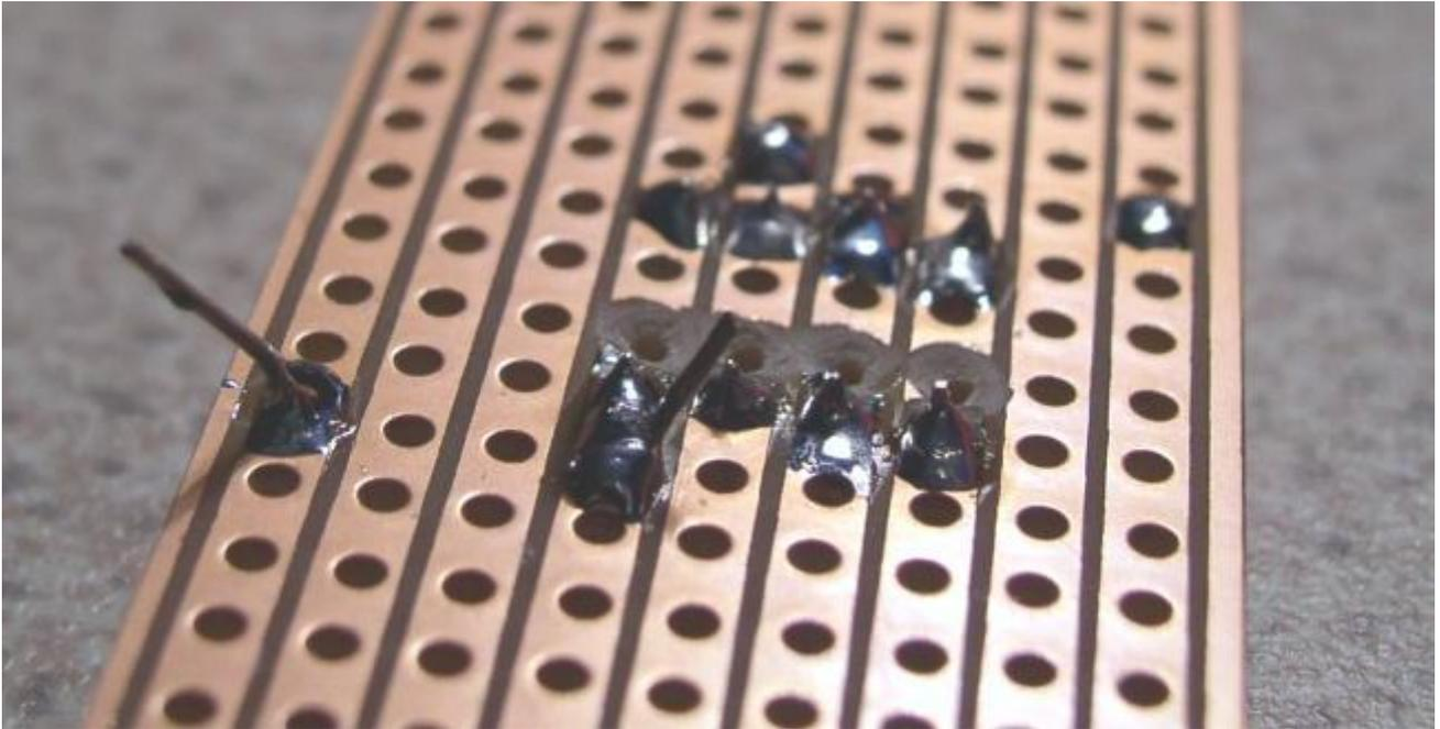
Components can be added in any order. Some people prefer to use the larger parts first, so that they are aware of the physical space left on the board. It is however good practice to solder veropins, jumpers first, then passive components, resistors, capacitors, inductors, followed by active components such as diodes and transistors next.
