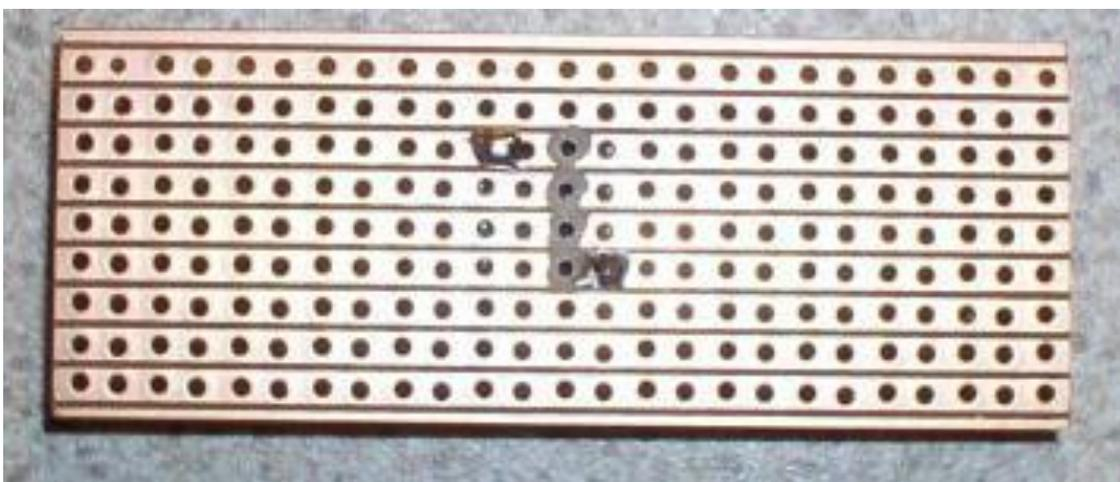
Diagonally opposite legs are first soldered. This makes sure the IC is held firmly. Next the veroboard track cutter is used to break 4 holes in the centre of the IC (or IC socket). Without this pins 1 and 8, 2 and 7, 3 and 6, 4 and 5 would be short-circuited. After breaking the tracks, solder the remaining pins on the IC or IC socket.
