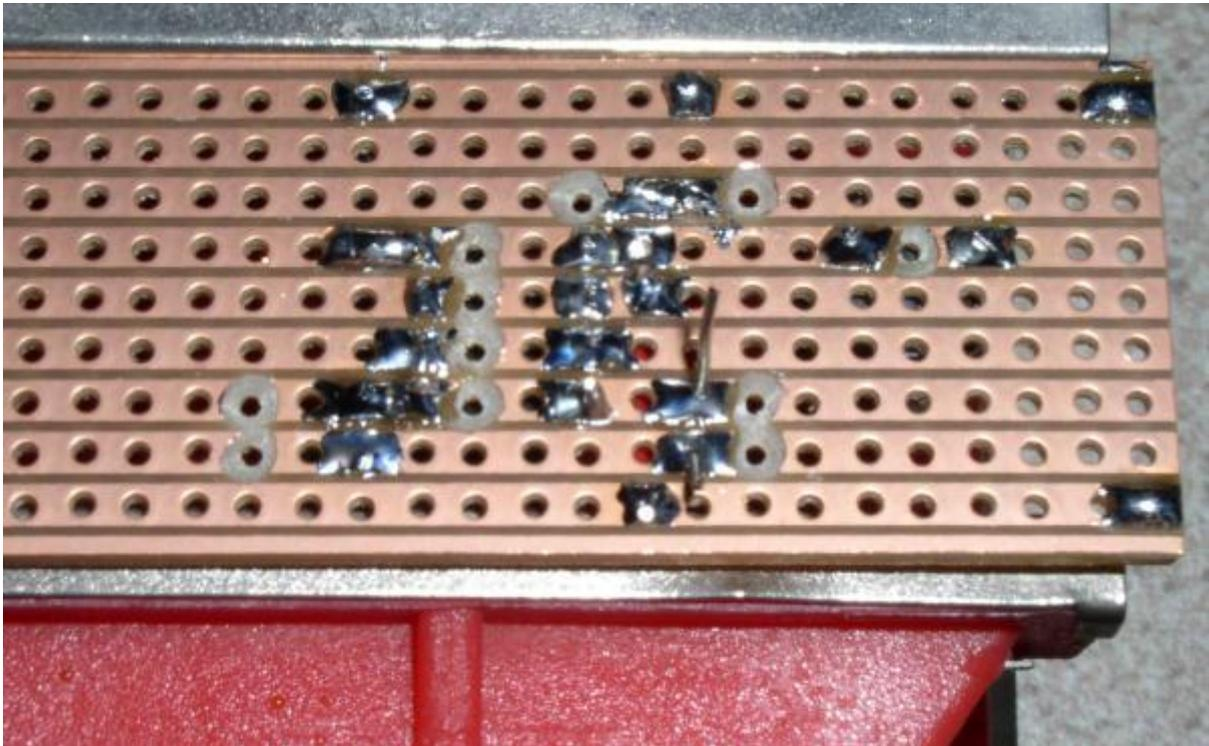
The blue jumper wire leads are shown (before being cut flush to the board). The 10uF capacitor is soldered and cut short. Note that the second track from the bottom is now connecting the negative side of the capacitor to the jumper wire which returns to the LM386 pin 8.
