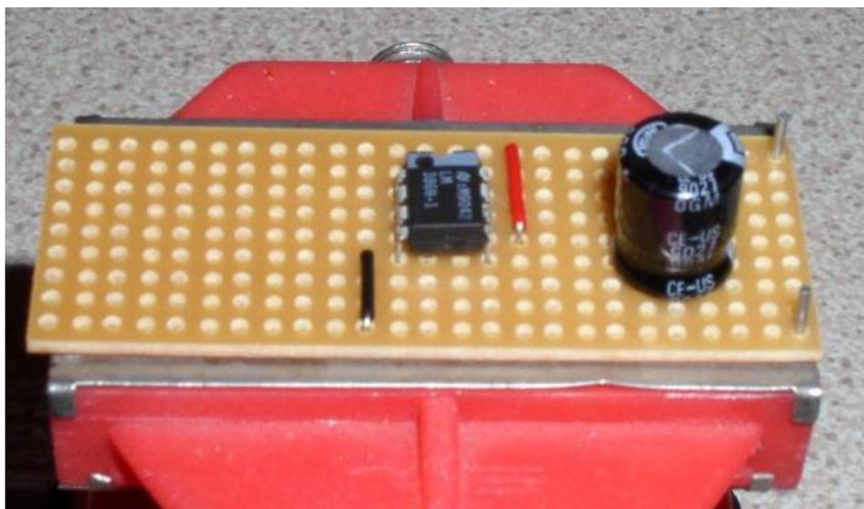
The board is turned over and the 330uF output capacitor put in place. From the schematic the "+" plate needs to connect to pin 5 of the IC. Place the
