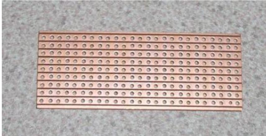
If a track is broken, with a drill bit or veroboard cutter, then you have two non-connected wires on the same horizontal strip. Note that NO continuity exists across adjacent tracks. If this should happen, i.e. when cutting a track and a piece of copper "swarf" should accidentally bridge two tracks, then the design would be compromised and probably not work at all. Therefore take care when breaking tracks and examine the board after making each break.
