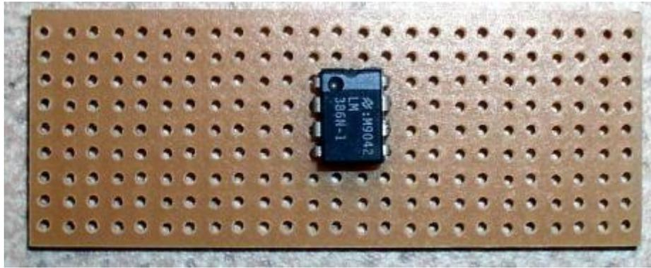
Look at the schematic. The triangle represents the LM386 Integrated Circuit component. As 7 connections are used it makes sense to place the IC somewhere central, (see above picture), as tracks above and below the IC will act as the wires for the power supply.
