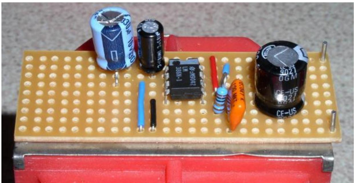
This capacitor is inserted so that the positive plate is on the positive power track and the negative plate reached to the same track as pin 2 of the LM386
